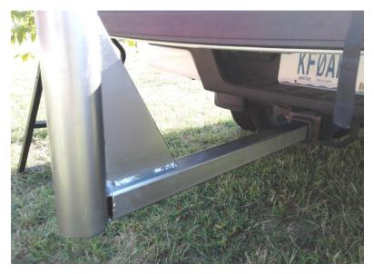
Don (KFØARQ) crafted this portable hitch mount antenna ... excellent for POTA events! The 2 inch square tubing is 31 inches long in order to clear the tail gate. The mast is an extendable 20 foot flag pole and supports a 20M dipole antenna.
